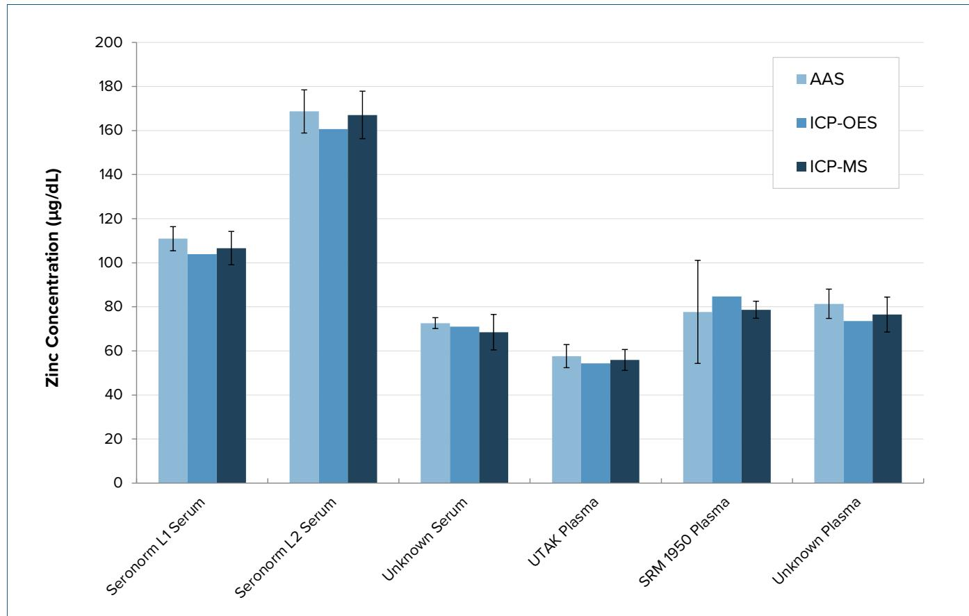
Zinc concentration of each serum and plasma sample was determined by AAS ( $n = 4$ ), ICP-OES ( $n = 1$ ), and ICP-MS ( $n = 4$ ). Data are displayed as mean  $\pm$  standard deviation. Standard deviation for ICP-OES is not calculated since only one such instrument was used. No differences were detected between AAS and ICP-MS for any material, or overall.
